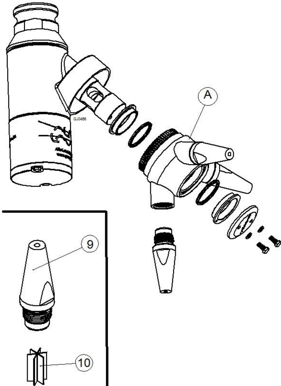
Drawing A6: Alfa Laval GJ 4 180° Directional Triple Nozzle Housing Assembly
