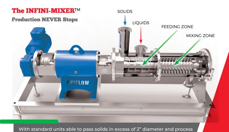
at temperatures up to 392°F, the Infini-Mixer™ can gently mix products up to 1,000,000cps. Product temperature is able to be tightly controlled by the use of jacketed housings and temperature regulated rotors.
