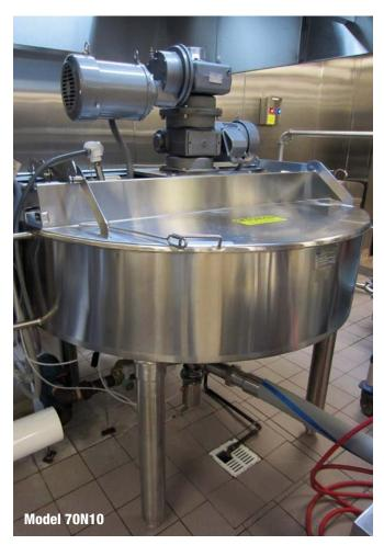
The heavy-duty agitator drive enables the scraper blades to rotate in one direction while the tri-blade center agitator, positioned deep within the vortex and powered independently of the scraper, turns in the opposite direction. This unique assembly together with the rugged fixed position baffle provides the operator with the capability to effectively combine and blend every conceivable assortment of ingredients and produce the most uniform and pleasing finished product possible.
