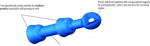
The waist of the lip pig enables the passing of  $90^{\circ}$  standard bends (R = 1,5 x D)
