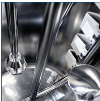
Triple Motion with Head B, Scrape, and Propellers
