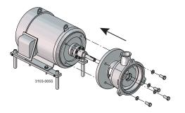
Step 6 1. Fit impeller (11) on stub shaft (3).
