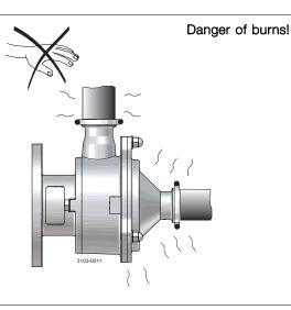
The pump and the pipelines must **never** be pressurised when the pump is serviced.
