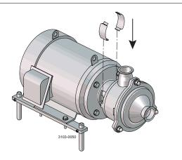
Study the instructions carefully. The items refer to the parts list and service kits section. Lubricate the rubber seals before fitting them.
