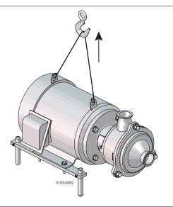
Study the instructions carefully and pay special attention to the warnings! The direction of rotation of the impeller can be checked by observing the direction of rotation of the motor fan. - See the indication label on the pump.
