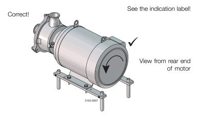
Study the instructions carefully and pay special attention to the warnings! The direction of rotation of the impeller can be checked by observing the direction of rotation of the motor fan. - See the indication label on the pump.
