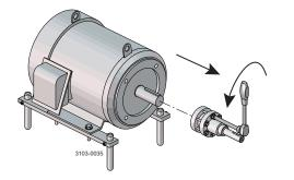
Step 12 Remove screws (5), washer (5a) and compression rings (4a+b) from stub shaft (3).
