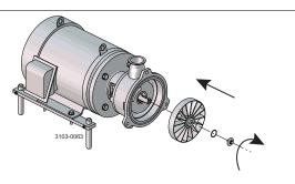
Study the instructions carefully. The items refer to the parts list and service kits section. Lubricate the rubber seals before fitting them.
