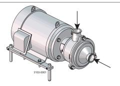
Step 3 Avoid damaging the inlet and the outlet.
