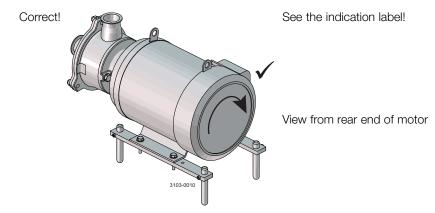
Study the instructions carefully and pay special attention to the warnings! The direction of rotation of the impeller can be checked by observing the direction of rotation of the motor fan. - See the indication label on the pump.
