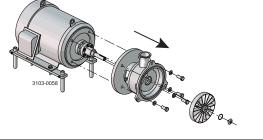
Study the instructions carefully. The items refer to the parts list and service kits section. Lubricate the rubber seals before fitting them.
