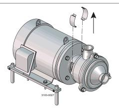
Step 2 Remove cap nuts (14), washers (15a) and casing cover (10).
