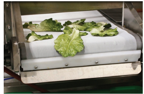
Automated ConveyORIZED Mesh Screen - Outside View
