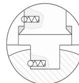
Pyramidal Stem, Double Sealing & Anti-Static Device
