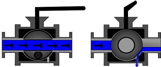
Vent to atmosphere is when the valve is open, product flows through the valve. No venting occurs because the vent passage is isolated from the flow path.
