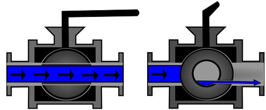
When the valve is open, system fluids flow through the valve. The vent passage allows pressure inside the valve to remain equal to system pressure.
