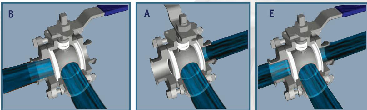
The **Tru-Flo** 3-way diverter port ball valve is designed to have the center port act as the common port and must be open at all times. You can use the L-port diverter to go from center to left (Fig. B) or to go from center to right (Fig. A). The T-port diverter can do the same configurations as the L-port but can also have all three ports opened at once (Fig. E).
