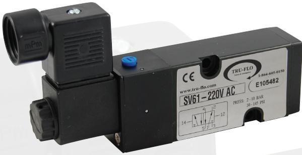
SV SERIES SOLENOID VALVE IS A COMPLETE RANGE OF VALVES DESIGNED ACCORDING TO NAMUR VDI/VDE 3845 AND MADE OF EPOXY COATED ANODIZED ALUMINUM. EACH SOLENOID VALVE IS FIELD INTERCHANGEABLE FOR USE ON EITHER DOUBLE ACTING 4-WAY OR SPRING RETURN 3-WAY ACTUATORS AND IS AVAILABLE IN SINGLE COIL, DUAL COIL, OR 3-POSITION CONFIGURATION (OPEN CENTERS, CLOSED CENTERS, OR CENTER IN PRESSURE).
