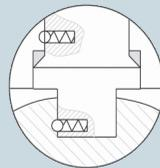
Pyramidal Stem, Double Sealing & Anti-Static Device
