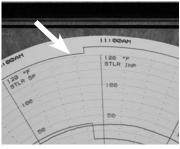
7. Expose HTST probe to a temperature above diversion setpoint – The forward flow (green) light should be on and the event line at the outside edge of the chart should be recording at the outer (forward flow) position.
