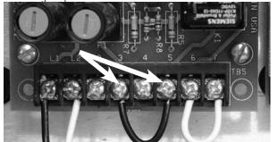
3. Install a second jumper wire from terminal 6 to terminal 7.
