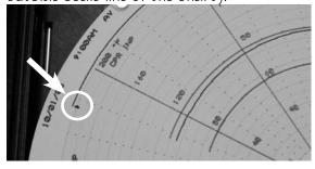
6. Expose HTST probe to a temperature below diversion setpoint – The divert flow (red) light should be on and the event line at the outside edge of the chart should be recording at the inner (divert) position.
