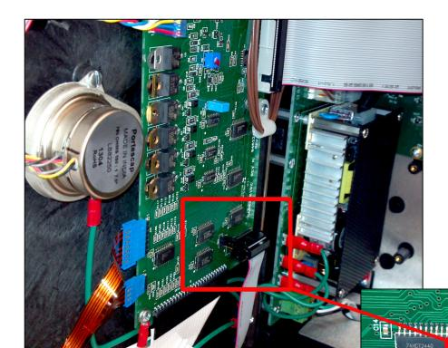
This jumper **MUST** be left in PROGRAM position at all times for AV-9900 Pasteurization Recorder Controller Units for proper operation.
