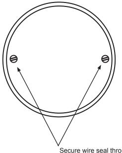
Secure wire seal through both screws to prevent removal of the backplate.
