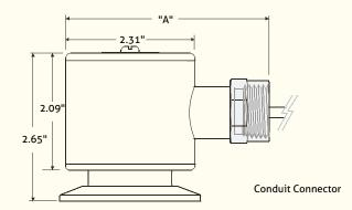
Optional: Sealed Cable with 1/2" NPT Conduit Connection
