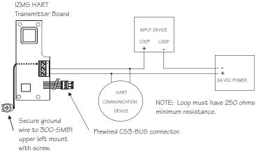
NOTE: Disconnecting the CS-3 terminal while operating the flowmeter will cause temporary lose of measurement.
