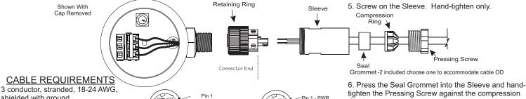
shielded with ground. 4-8mm (0.16-0.31") Cable Sheath OD.
