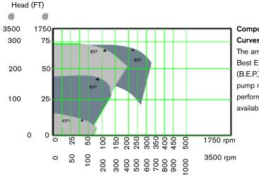
Composite Performance Curves for the V<sup>2</sup> Series The arrows indicate the Best Efficiency Point (B.E.P.) for various pump models. Individual performance curves are available upon request.
