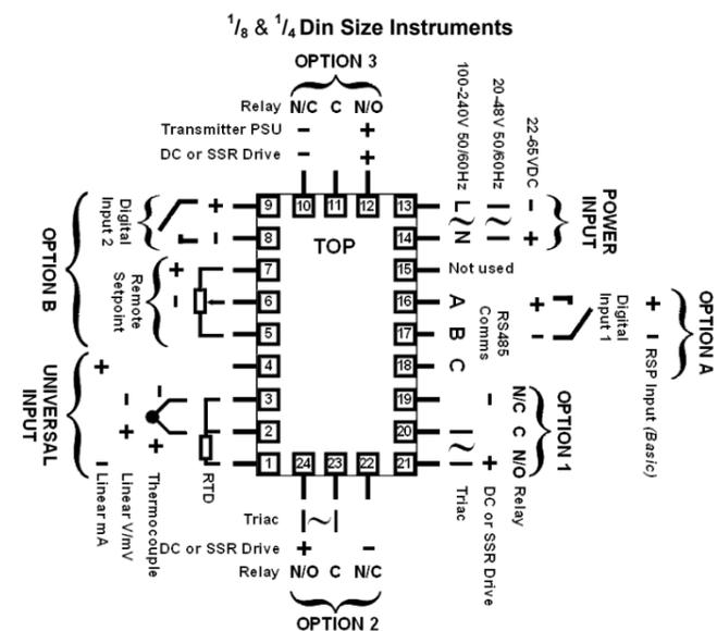
**Note:** These diagrams show all possible option combinations. The actual connections required depends on the exact model and options fitted.
