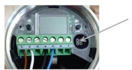
Connection plug for the MPI-200-F adapter as an intermediate plug between the ITM-51 electronics and the MPI-200 connection 3 (see the next figure).
