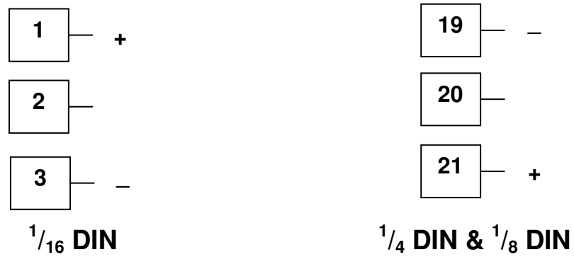
Figure 22. Option Slot 1 - Linear Voltage &amp; mADC Module
