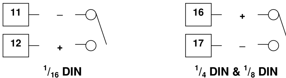
Figure 33. Option Slot A – Digital Input Module
