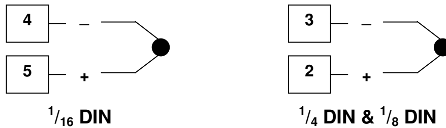
Figure 16. Thermocouple Input Connections
