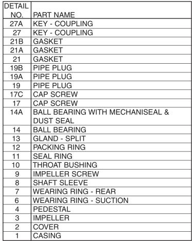
NOTE: Please be sure to always include pump type, size, and serial number with any reference to above numbers and names.
