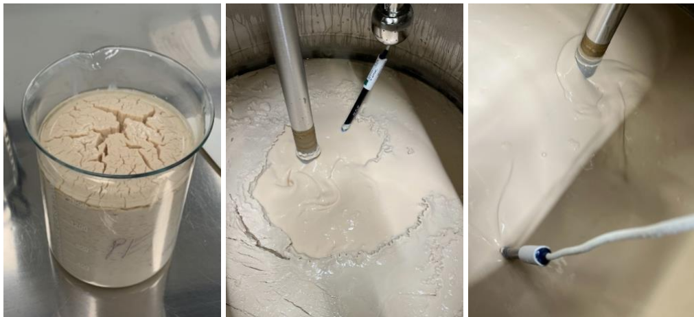
Figure 11 To the left a coagulum from laboratory trials without agitation. The image in the middle shows the results of insufficient agitator speed during fermentation. The right image reflects sufficient agitation throughout fermentation
