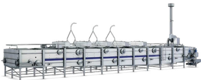
Fig. 16.23 Salting mellowing conveyor.
