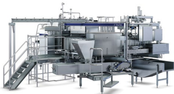
Fig. 16.29 Rotary moulder chiller (moulding machine for pizza cheese).
