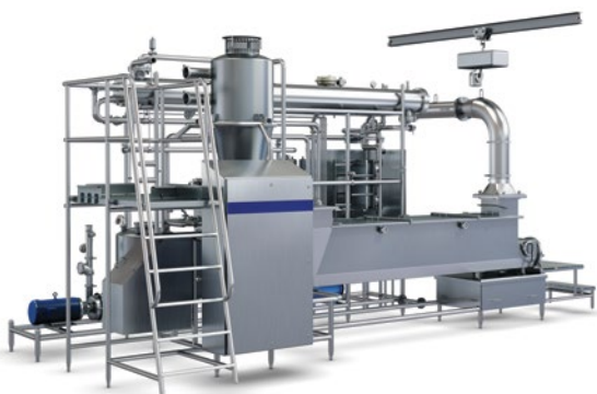
Fig. 16.28 Continuously operating cooker-stretcher for pasta filata types of cheese.
