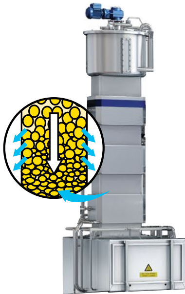
Fig. 16.19 Whey is drained through the perforated sections on the column.
