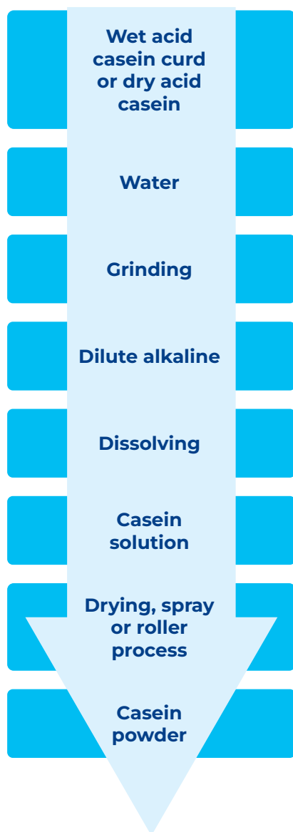
Fig. 16.48 Basic steps involved in the manufacture of spray or roller-dried caseinates from acid casein curd or dry acid casein. Alkali may be sodium hydroxide, potassium hydroxide, calcium hydroxide, or ammonia.
